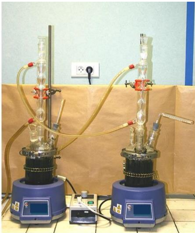
Figure 2.16 Example of testing equipment available on the market to perform UN Test C.1
