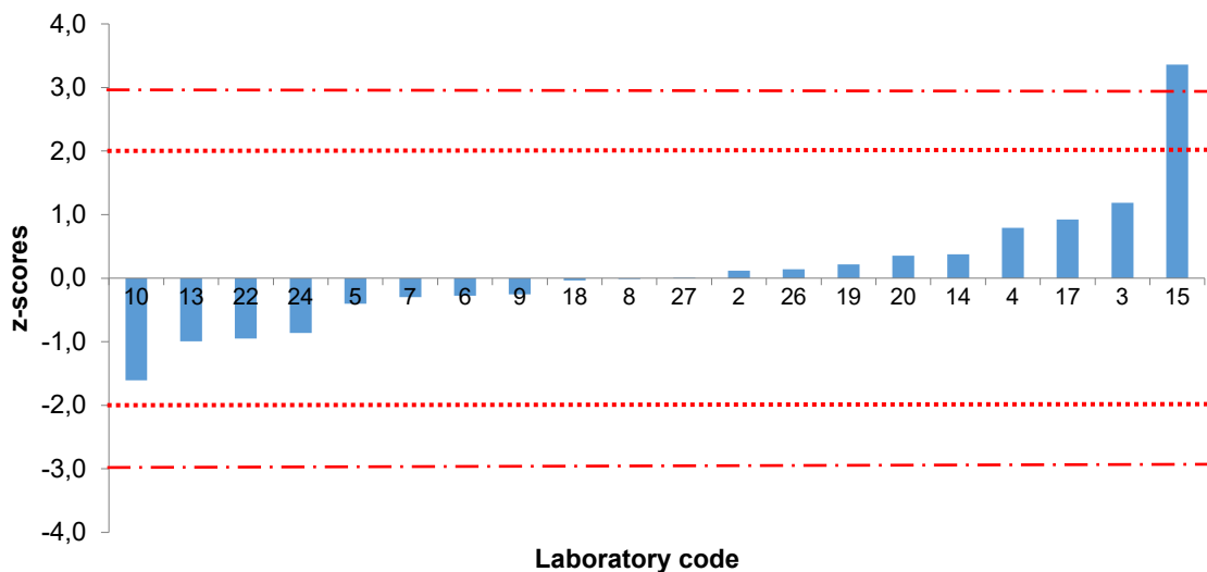
Figure 12. Afs; z-score values (assigned value x \pm U(x) = 1.84 \pm 0.20 \mu\text{g}/\text{kg} ; \sigma_p = 0.46 \mu\text{g}/\text{kg} ). PT 2025 AFs in pistachios
