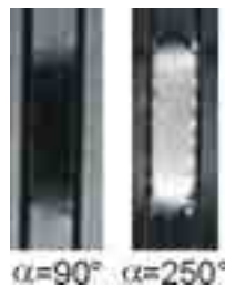
Figure 2. Flip-angle signal dependence within the lumen (Reprinted with permission of Wiley/Liss, Inc., a subsidiary of John Wiley & Sons, Inc.) (9)
