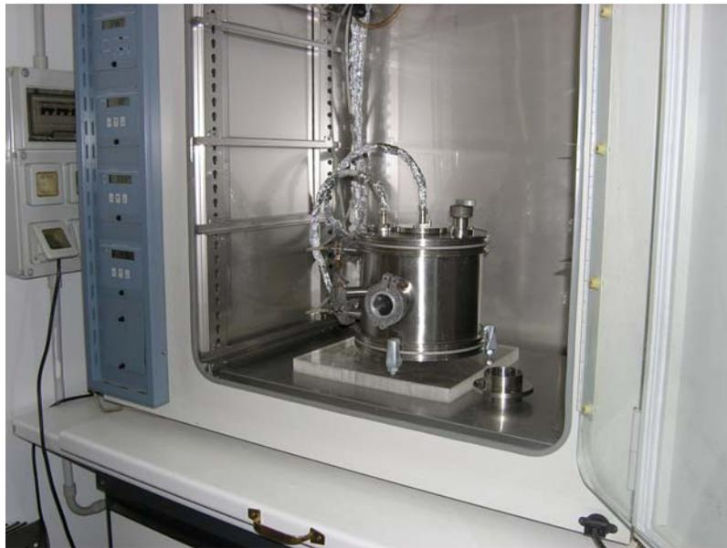
Figure 3. The alpha-irradiator placed into a standard CO<sub>2</sub> incubator
