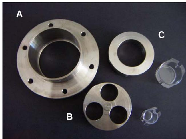
**Figure 2. Stainless steel Petri dish (A) designed for the alpha-particle irradiator (~25 cm<sup>2</sup> useful area), able to allocate the companion dishes B or C for experiments with inserts**
