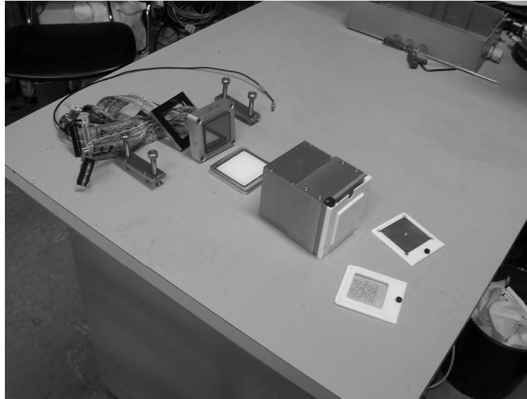
Figure 1. One of the detector systems used, based on a flat panel PSPMT. Collimation masks can be seen to the right of the detector box
