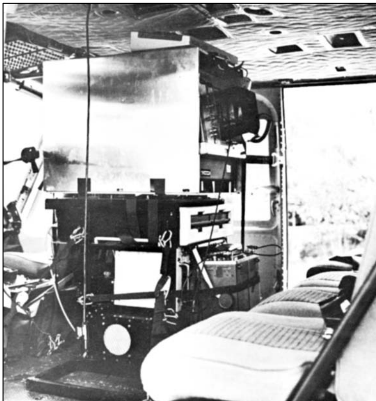
Figure 5. The bulky control system hosted on Agusta-Bell 412 helicopter
