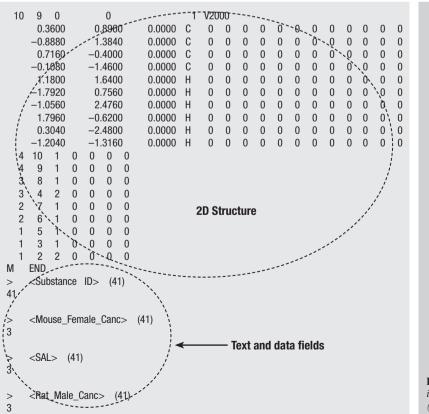
**Fig. 1** | A sample SDF file, containing both structural (top) and data (bottom) information.
