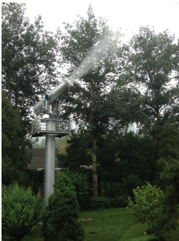
Figure 1 Application of a Fog-cannon placed at the Italian Embassy in Beijing (Sanlitun).
