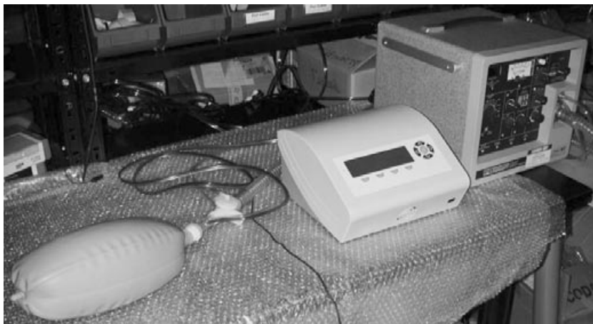
Fig. 5 | Experimental setup for testing of the ventilation board (respiratory balloon, our instrument, a commercial pulmonary ventilator, from left to right, respectively).
