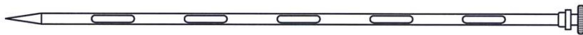
Figure B.2 — Open shaft with several apertures or closed shaft with compartments and several apertures
