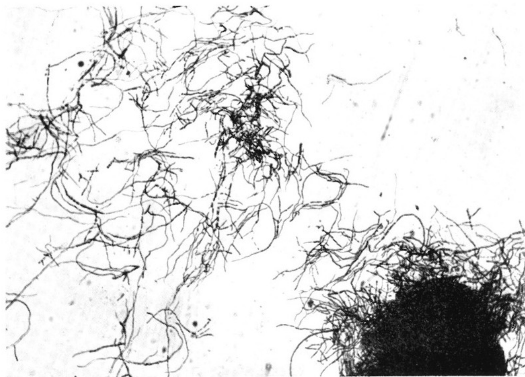
Fig. 8. - Long, filamentous mycelium and pellet after 47 hours growth in 12000 litre fermenter. (Baffled system, 160 r.p.m., 600 mm \phi ) \times 150.
