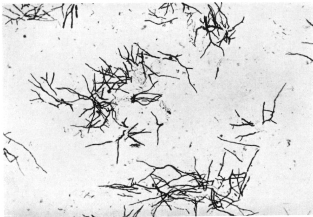
Fig. 11. - Short branched mycelium after 72 hours growth in 3000 litre fermenter with vigorous agitation. (Vortex system, 760 r.p.m., 350 mm \phi ) \times 225.
