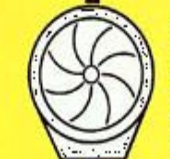
SCOURER—beaters in screen cylinder scour off impurities and roughage.
