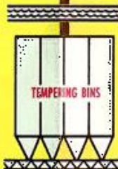
TEMPERING—water toughens outer bran coats for easier separation—softens or mellow endosperm.
