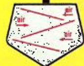
ASPIRATOR—air currents remove lighter impurities.
