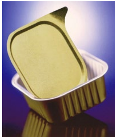
Figure B7.11.d. Typical PET-food container lacquered outside; laminated with CPP inside with thermo-sealable lid (inside CPP coextruded and outside lacquered and, possibly, printed)
