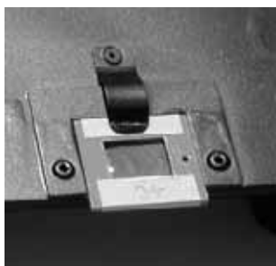
Figure 2. Polysulphone dosimetry device for the study of the distribution of UV radiation on the human body
