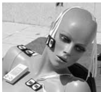
Figure 2. Polysulphone dosimetry device for the study of the distribution of UV radiation on the human body
