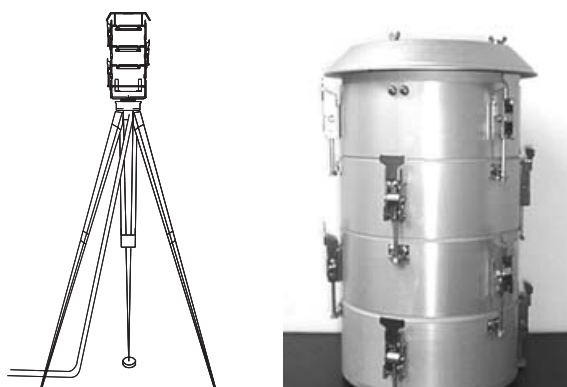
Fig. 5. - Schematic diagram and picture of the high volume cascade impactor.
